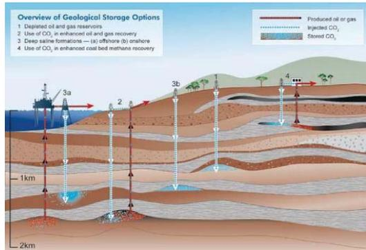
Fig. 4. The Conceptual Diagram of CCS.
