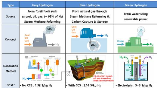
**Fig. 1.** Hydrogen Production Methods.
